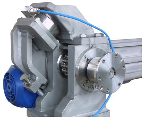
The felt / wire line adjustment in the TC stretch-compensators is carried out by a screw-jack which limits the adjustment field of the roll and at the same time measures its misalignment. This adjustment can be manual or motorized and the measure of misalignment can be visual or remote-controlled for the sections of machine which are less accessible.
